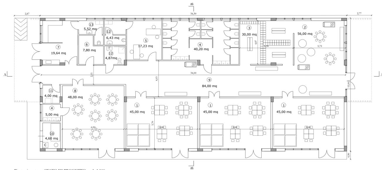
Pianta piano terra\_STATO DI PROGETTO\_scala 1:100
